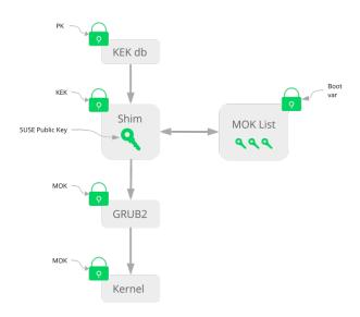
FIGURE 11.2: UEFI: SECURE BOOT PROCESS
