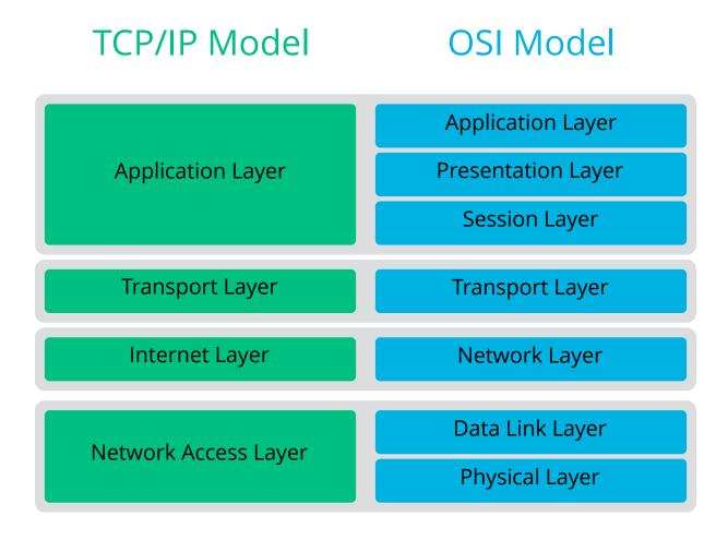
FIGURE 16.1: SIMPLIFIED LAYER MODEL FOR TCP/IP
